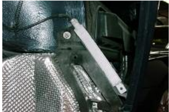
Antenna location in wheel well
